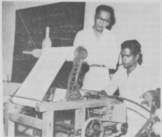
Fig. 3 - A trainee at the Fishing Gear Research Station in Cochin learns to use a net-making machine under the instruction of a fishing gear technologist.
