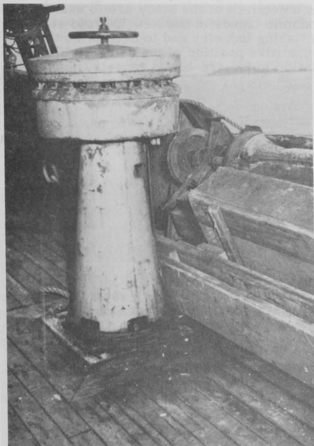
Fig. 8 - Fairlead and capstan used to haul the footrope aboard. This gear is mounted near the vessel's bow on the starboard side.
