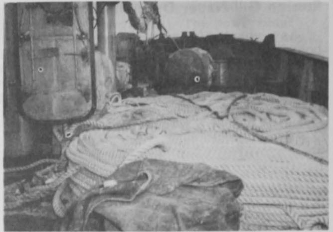
Fig. 6 - Footrope of gill net coiled on starboard side of vessel. The heavy footrope provides the weight to sink the nets. It is suspended from the gill net by rings similar to those on a purse seine.
