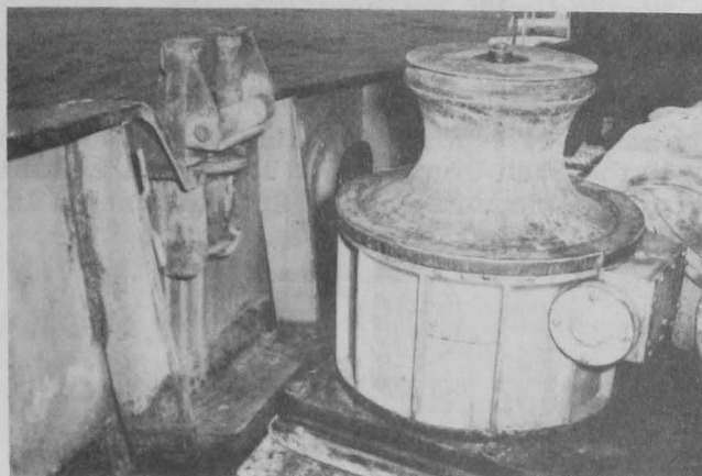
Fig. 8 - Fairlead and capstan used to haul the footrope aboard. This gear is mounted near the vessel's bow on the starboard side.
