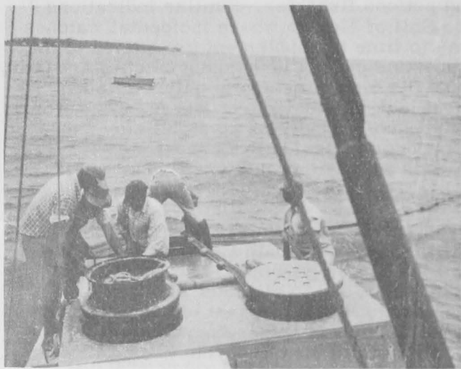
Fig. 2 - The Florida lampara-seine operation for sardines. The two wings of the lampara are being brought aboard with the aid of a two-roller gurdy.
