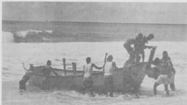
A 20-foot aluminum surf boat designed and built in England for the Nigeria Fisheries Department. It is an experimental vessel designed under Food and Agriculture Organization guidance for ring-net fishing. Shows the rudder being placed in position during the first trials of the boat.
