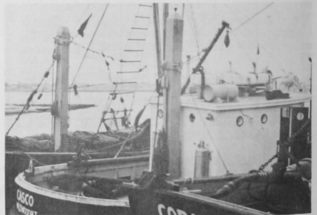
Fig. 4 - The towing bit is set from the keel and is high enough to allow the dredge towline to pass clear of the stern. The towline is reeved through a snatch block that is fastened to the towing bit before holding turns are applied to reduce chafing of towline. Hose used for jetting measures 5 inches in internal diameter and is constructed of heavy-duty collapsible nylon-reinforced rubber. Sections of the hose (seen along the rail) are fastened together with pressure clamps over aluminum sleeves. The hose is always longer than the towing warp.
