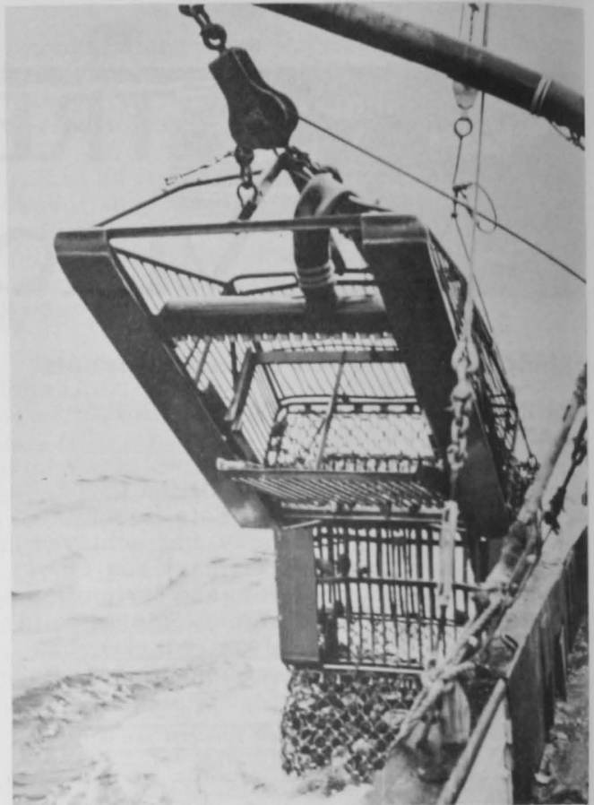
Fig. 2 - Hydraulic Jet Dredge. Dredges consist of two basic parts, the dredge section proper and the sled section. The dredge section (forward) has a manifold of 5- or 6-inch pipe with a series of horizontally-spaced nozzles aimed down, back, and immediately forward of the cutting knife. Water pressure is maintained at about 70 pounds with a volume of from 1,000 to 1,500 gallons per minute. The sled section is attached to the dredge section to retain the clams washed back from the dredge.
