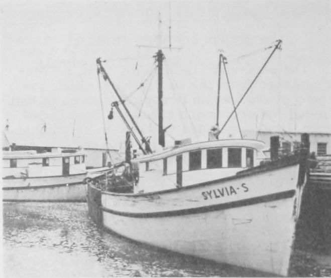
Fig. 1 - A typical Diesel-powered surf-clam vessel. Vessels in use range from 65 to 90 feet in length. An auxiliary Diesel engine is mounted below deck, aft, to drive a 5-inch centrifugal pump that supplies water for the hydraulic dredge.
