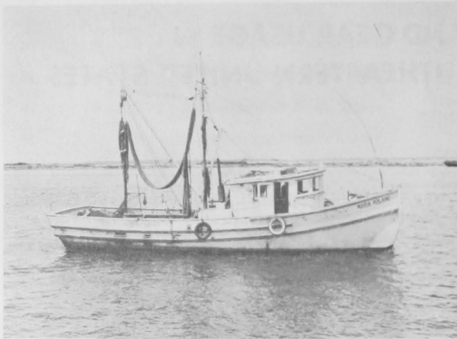
Fig. 2 - A typical single-rigged "Florida-type" shrimp trawler. The single net is dragged from the starboard boom. The smaller port boom or "outrigger" is used to drag a small trynet.
