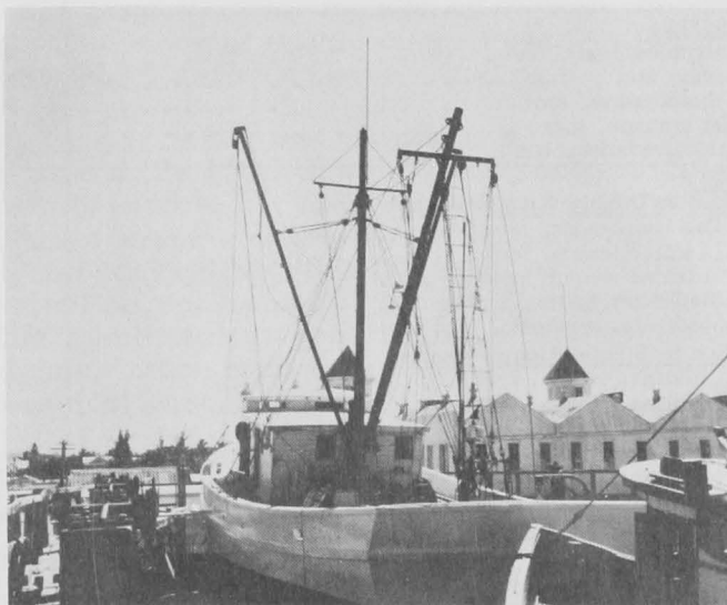
Fig. 1 - A typical double-rigged "Florida-type" shrimp trawler. At sea, the "outriggers" or port and starboard booms are lowered and one trawl is dragged from each.
