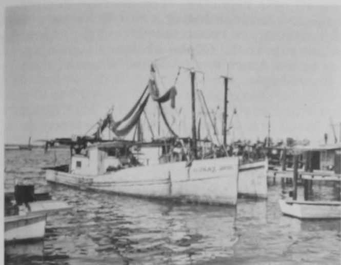
Fig. 3 - "Biloxi-type" shrimp trawlers. The single net is dragged a-stern from warps leading over blocks at the after corners of the house.
