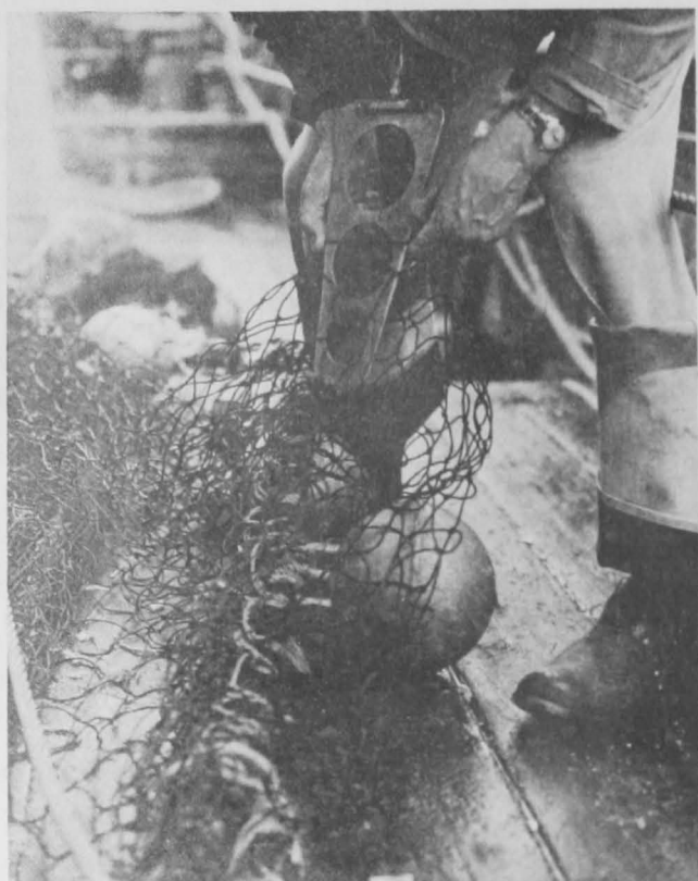
Instrument used to take internal mesh measurements (M/V Delaware Cruise 61-6).
