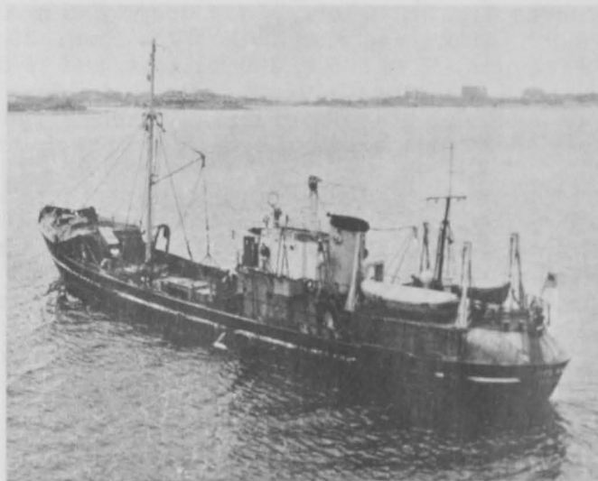
Fig. 1 - The M/V Delaware , a conventional, steel-hulled North Atlantic otter trawler with a displacement weight of 518 tons and a length of 147.5 feet, is rigged for side fishing. The Bureau-owned vessel is used for exploratory fishing and gear research by the Gloucester, Mass., Exploratory Fishing and Gear Research Base.
