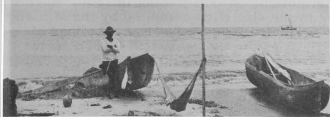
Wood fishing boats carved from a single trunk on Richacha Beach, Colombia.
