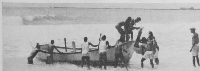
A 20-foot aluminum surf boat designed and built for the Nigeria Federal Fisheries Department in 1956. An experimental vessel for ring-net fishing. Rudder being placed in position prior to sailing for its first trials.
