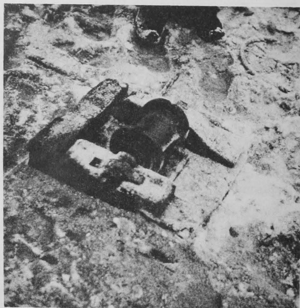
Portable roller for beaching smaller Danish fishing boats.
