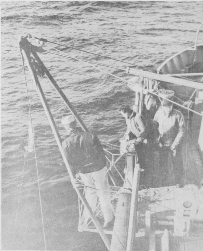
Fig. 1 - Nansen bottle used with oceanographic winch to obtain water samples and temperatures at any depths aboard a Coast and Geodetic survey ship.
