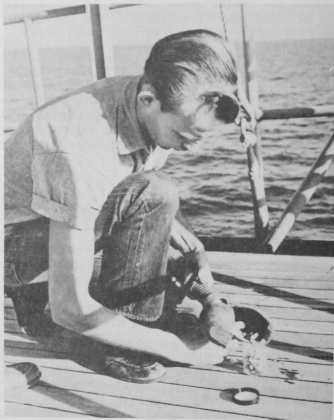
Fig. 2 - Sea bottom sampler snapper used aboard a Coast and Geodetic survey ship.
