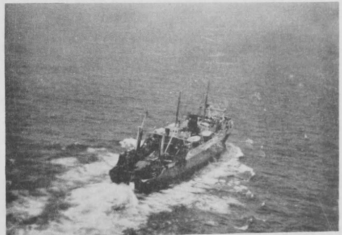
Russian factory-type stern trawler fishing on northern edge of Georges Bank. Length about 300 feet.
