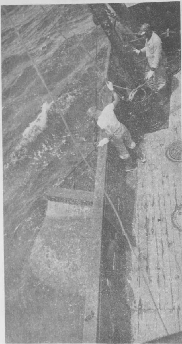
Fig. 2 - Hauling back a Georges Bank scallop dredge.
