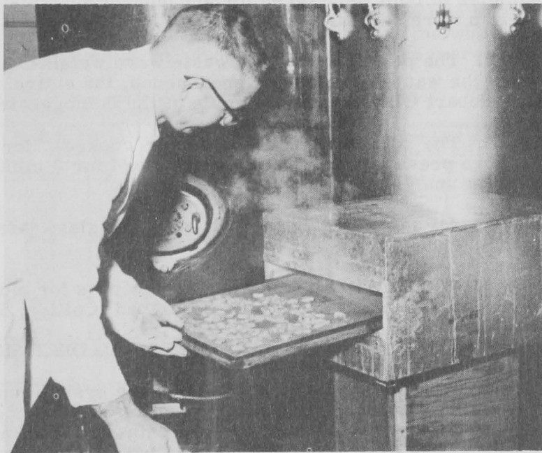
Fig. 1 - Chemist preparing to precook raw peeled shrimp in the laboratory steam box.
