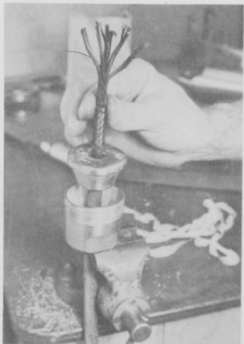
Fig. 10 - Operation 10. Remove the glass tape. Roll back and carefully cut off the nylon sheath covering the conductor section. Separate the conductors and the fillers. Cut away the fibrous fillers and the rubber center filler. Cleanse the conductors with a rag dampened in solvent.
