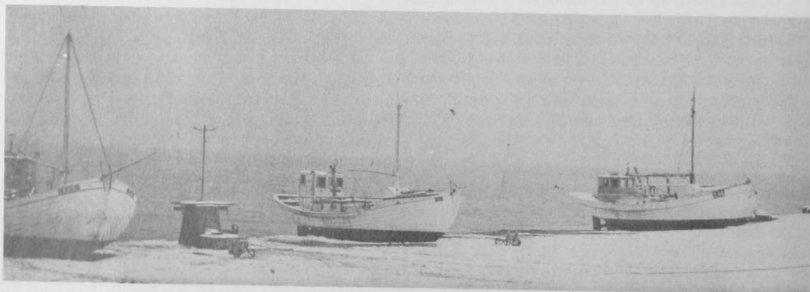
Large Danish beach-landing fishing craft which are both launched and hauled ashore with the help of large electrical winches. In Denmark many fishing craft are landed direct onto beaches.
