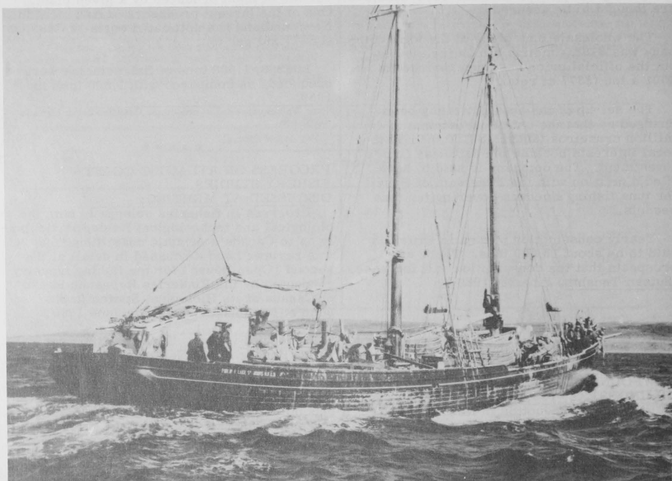
Canadian east coast schooners, equipped with Diesel or gasoline engines, fish for cod and other groundfish. Fishermen use dories to catch fish with hook-and-lines. Sail is only auxiliary.
