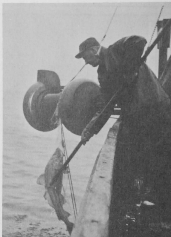
Fig. 2 - Cod being hauled aboard over the fairlead drum. The crewman is one of five aboard the vessel. Hauling of the gear is usually started at daybreak and takes 2 to 3 hours.
