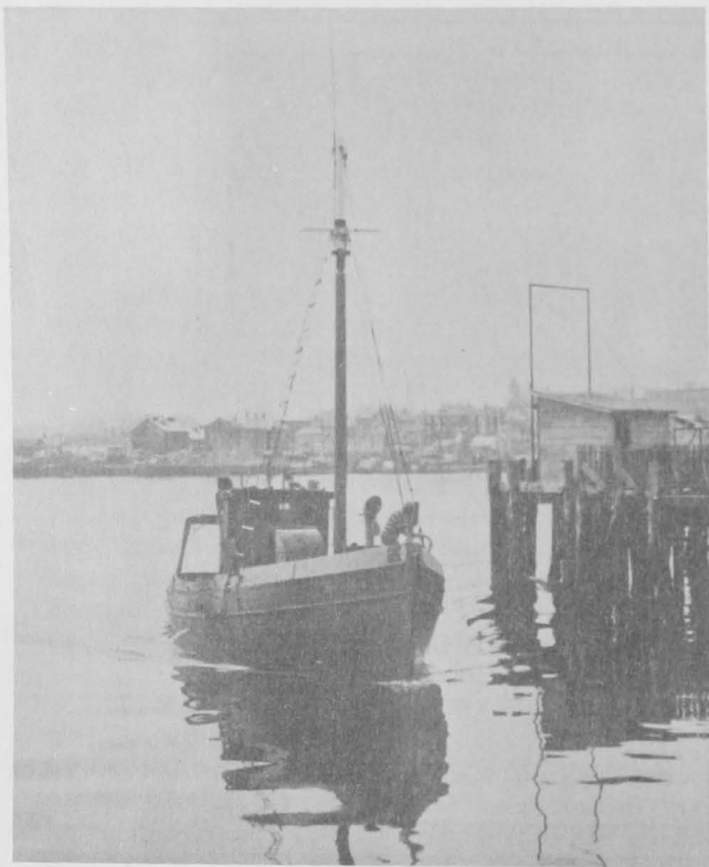
Fig. 1 - The Phyllis A. , a 55-foot Gloucester vessel engaged in the sink gill-net fishery. The vessels in this fishery vary in length from 55 to approximately 75 feet. Practically all of the fishing takes place within a 30-mile radius of Gloucester.
