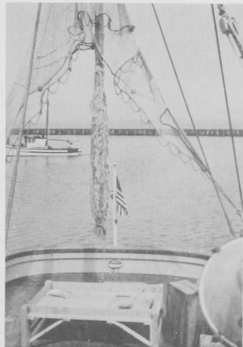
Fig. 2 - A 43-foot Gulf of Mexico-type shrimp trawl drying in the rigging of the M/V John N. Cobb . The sorting table is shown below the net.
