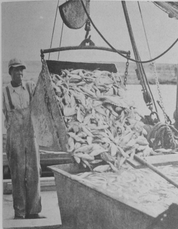
Fig. 2 - Dumping fish into tanks at beginning of conveyer line at a Gulf of Mexico plant using industrial fish in canned pet food.
