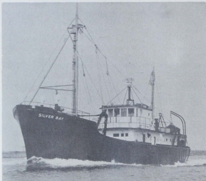
Fig. 6 - M/V Silver Bay --a 96.4-foot New England-type side trawler used to terminate royal-red shrimp explorations along the South Atlantic Coast.
