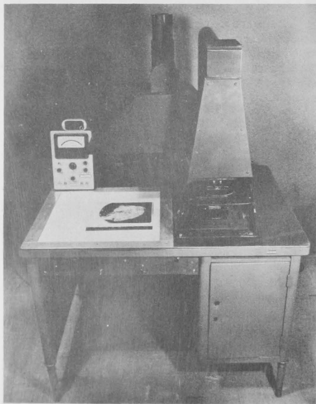
Fig. 7 - Electro-optic scale reader accurately, rapidly, and semi-automatically provides data on individual salmon scales.
