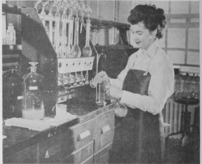
Fig. 2 - Crude protein content of fish scales is determined by Macro-kjeldahl procedure.
