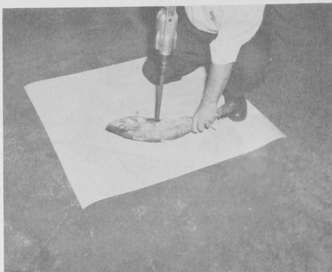
Fig. 3 - Sampling frozen haddock with rotary core sampler.
