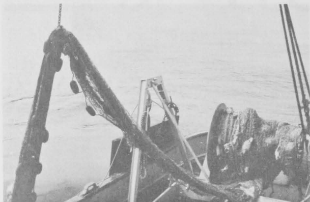
Fig. 7 - The fish bag alongside ready for splitting. Note how, after splitting, the intermediate trawl section and bag are wound directly onto the trawl drum without further handling or vessel maneuvering.
