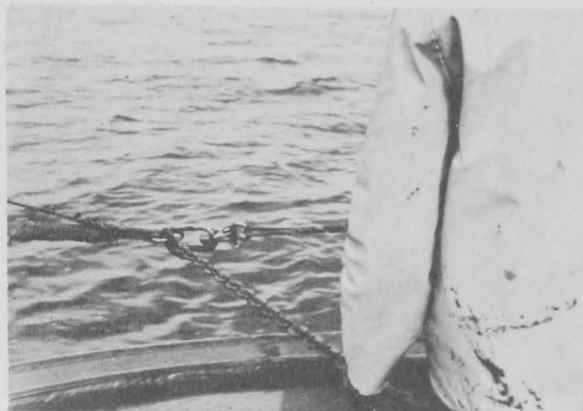
Fig. 5 - The dandyline (on the other side of the fisherman) has been reeved through the davit towing block and connected to the trawl bridle. When the dandyline receives the strain of the gear, the stopper chain will be disconnected. Note the G-hook at the end of the dandyline.
