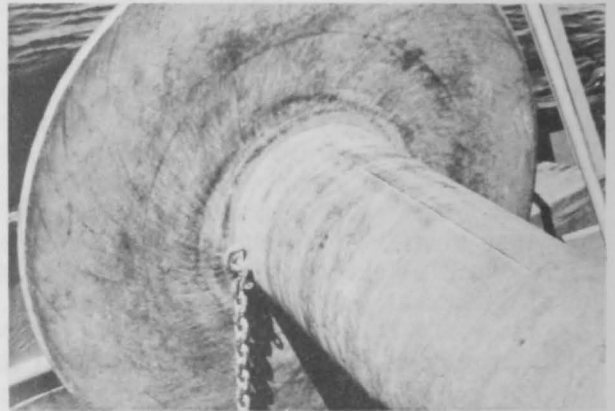
Fig. 2 - Stopper chain. A six- to seven-foot stopper chain is secured near each end of the core of the trawl drum. A snap is secured to the other end of the chain to receive the bridle.
