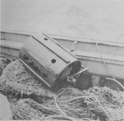
Fig. 3 - The "lawn roller" meter used to measure the distance traveled by the trawl on the bottom-- developed by the Fisheries Instrumentation Laboratory, U. S. Fish and Wildlife Service, Seattle, Wash.
