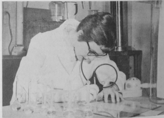
FIG. 1 - PAPER PARTITION CHROMATOGRAPHY IS USED TO IDENTIFY UNKNOWN AMINO ACIDS IN PROTEIN HYDROLYSATES.
