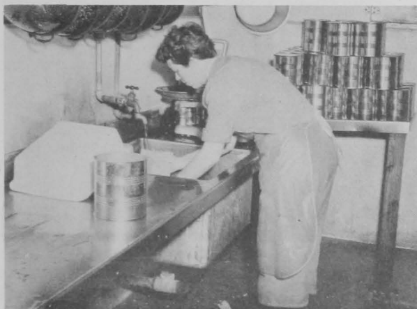
FIG. 33- WASHING CRAB-PROCESSING EQUIPMENT AFTER USE. PROPER SANITATION IS OF UTMOST IMPORTANCE IN MAINTAINING THE QUALITY OF CRAB MEAT. IN THE BACKGROUND ARE THE NO. 10 CANS THAT ARE USED AS CONTAINERS FOR FRESH VACUUM-PACKED CRAB MEAT. EACH CAN HOLDS 5 POUNDS OF CRAB MEAT WHEN FILLED AND SEALED. THE SEALED CANS ARE CHILLED, HELD, AND SHIPPED IN CRUSHED ICE.
