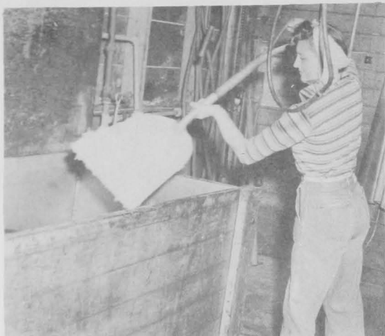
FIG. 18 - ICING SALMON. IN THIS CASE, THE SALMON ARE BEING ICED IN A STAINLESS-STEEL VAT, THE OTHER CONTAINERS BEING FULL AT THE MOMENT. UNLESS PROPERLY CHILLED WITH ICE, FISH BEGIN TO SPOIL IMMEDIATELY.
