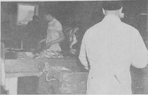
FIG. 27 - WORKER IN THE RIGHT FOREGROUND IS KILLING CRAB, THE FIRST STEP IN THE PROCESS FOR OBTAINING CRAB MEAT. ONLY LIVE CRABS ARE USED IN ORDER TO INSURE THE FRESHNESS OF THE FINAL PRODUCT.
