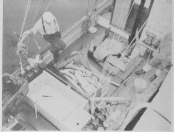
FIG. 10 - BOX AND GEAR USED BY FISH-BUYING FIRM TO LIFT TROLL-CAUGHT SALMON FROM THE TROLLER TO THE DOCK, NOTE THE IMMACULATE CONDITION OF THE TROLLER. THE CARE WITH WHICH FISH ARE HANDLED ABOARD THE VESSEL CONTRIBUTES VERY GREATLY TO THE QUALITY OF THE PRODUCT.
