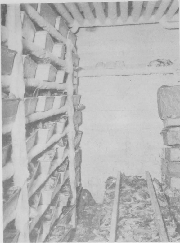
FIG. 37 - PANS OF FISH ON THE SHELVES OF A SHARP FREEZER. GREAT CARE IS TAKEN TO INSURE THE ABSOLUTE FRESHNESS OF THE MINK FEED.
