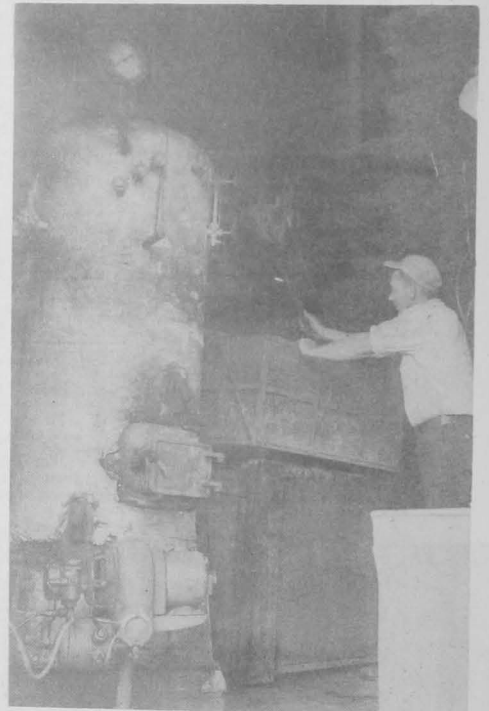
FIG. 30 - REMOVING COOKER BASKET FROM STAINLESS-STEEL-LINED COOKER VAT. NOTE OVERHEAD TROLLEY AND ELECTRIC BLOCK FOR LIFTING.
