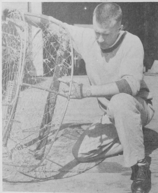
FIG. 21 - IRON BAR PROVIDES FOR WEIGHT AND ALSO ACTS AS A SACRIFICIAL ELECTRODE TO PRESERVE THE POT FROM CORROSION.
