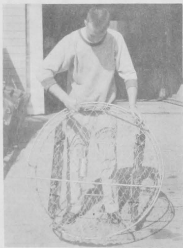
FIG. 20 - NEW STAINLESS-STEEL CRAB POT CONSISTING OF FRAME, WIRE NETTING, IRON WEIGHTS, AND BAIT CAN. A CRAB POT SHOULD WEIGH ABOUT 100 TO 110 POUNDS TO KEEP TIDES AND CURRENTS FROM CARRYING IT OVER THE OCEAN FLOOR. EVEN POTS WEIGHING 110 POUNDS WILL SOMETIMES BE MOVED AS FAR AS 2 TO 10 MILES IN A SINGLE STORM.
