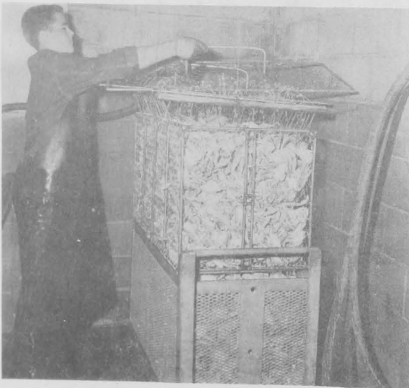
FIG. 31 - COOKING CRABS IN A SPRAY OF COLD FRESH WATER. CRABS ARE COOLED FOR 10 TO 15 MINUTES.
