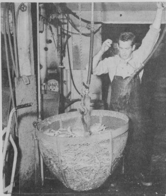
FIG. 23 - STAINLESS-STEEL BAIT CAN. CLAMS ARE THE PREFERRED BAIT.
