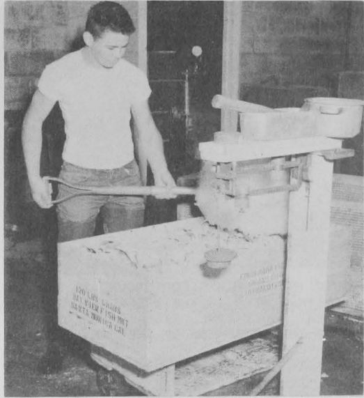
FIG. 25 - ICING WHOLE-COOKED CRAB IN WOODEN BOXES FOR SHIPMENT TO THE RETAIL MARKET. THE UPPER SHELL OF THE DUNGENESS CRAB IN THE NATURAL STATE IS A DARK BROWN OR PURPLE, WHICH CHANGES TO RED DURING COOKING. THIS SHADE OF RED REGISTERS ALMOST WHITE ON THE PHOTOGRAPHIC FILM USED.
