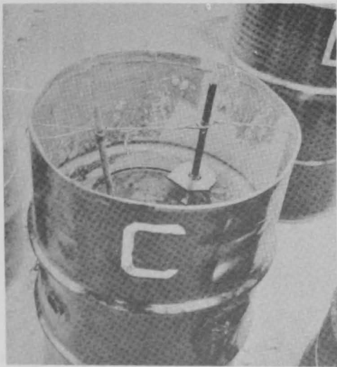
Copper tube pressure release is on the left.
