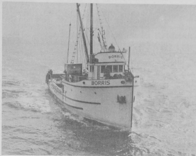
Fig. 3 - A trawler of the type that could be used in an Alaskan commercial fishery for Pacific ocean perch. Note the otter-trawl boards at the stern of the vessel.
