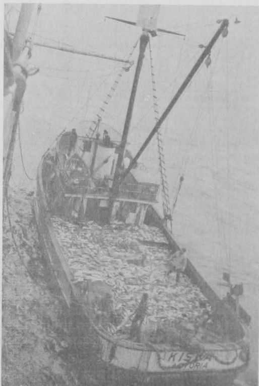
Fig. 4 - View of otter trawler from the stern with a deckload of fish.
