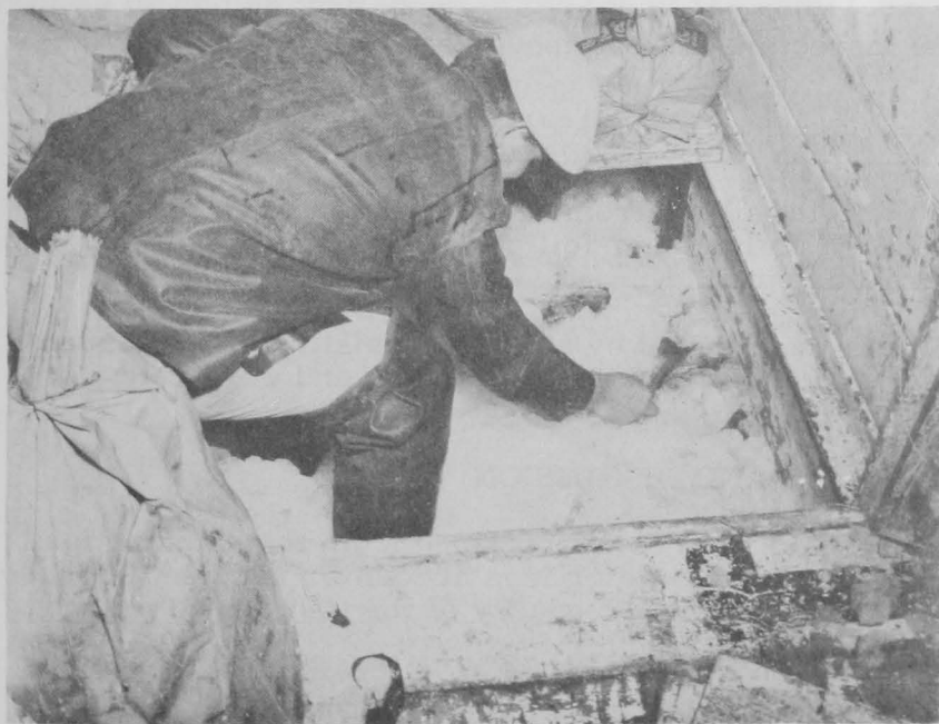
FIG. 5 - CHECKING THE TEMPERATURE OF THE HADDOCK WITH A MERCURY THERMOMETER.
