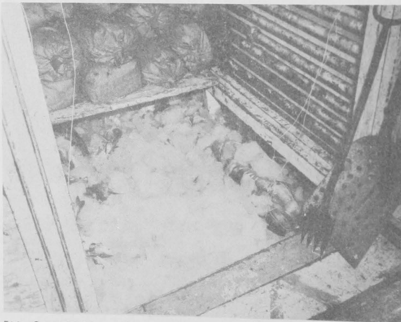
FIG. 3 - HADDOCK ICED IN THE PENS OF THE VESSEL WITH FRESH-WATER ICE. NOTE THE THERMOCOUPLE WIRES LEADING TO THE INDIVIDUAL FISH.
