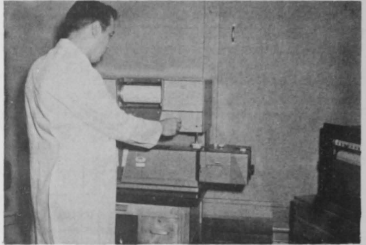
Fig. 1 - Measuring activity of a glycolytic enzyme by spectrophotometric assay.
