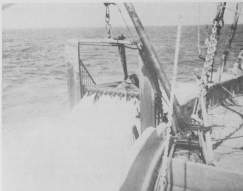
Fig. 1 - Dredging equipment being hauled in aboard the U. S. Bureau of Commercial Fisheries chartered vessel Sunapee .
