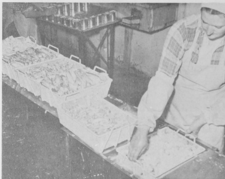
Fig. 6 - King crab meats being given a citric acid bath prior to canning.
