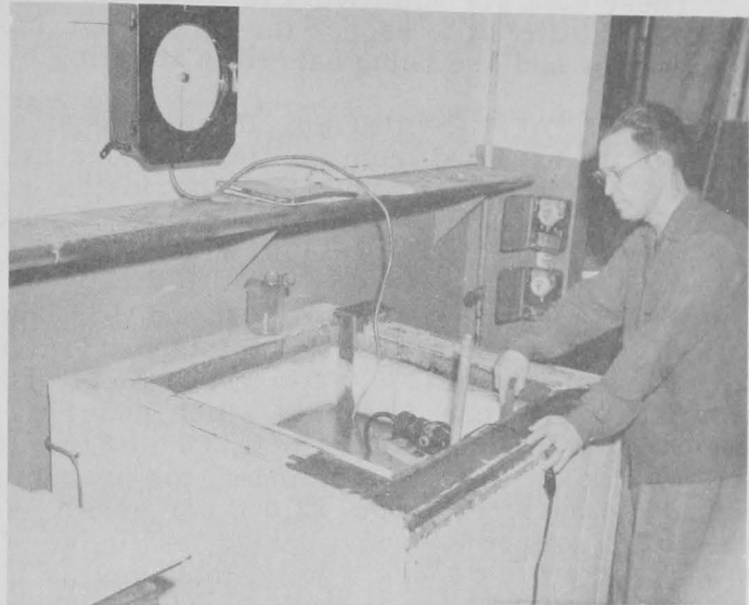
Fig. 5 - Experimental freezing tank used for pilot-scale experiments to determine time required to freeze round fish in refrigerated brine prior to sea experiments aboard the research vessel Delaware .
