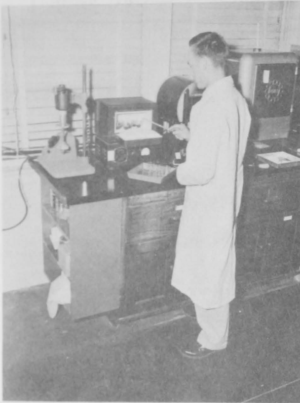
FIG. 1 - ASHING A SAMPLE OF FISH BY MEANS OF ELECTRIC FURNACE.
