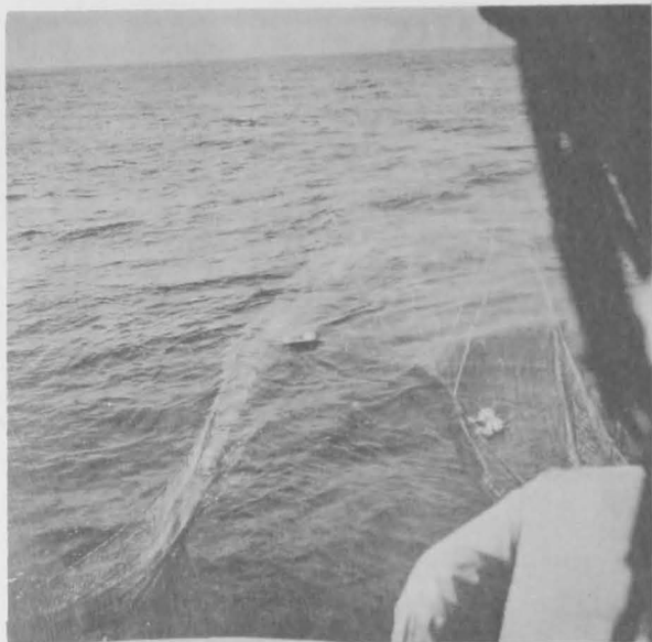
FIG. 2 - THE CANADIAN-TYPE MIDWATER TRAWL BEING SET FROM THE STERN OF THE METACOMET .
