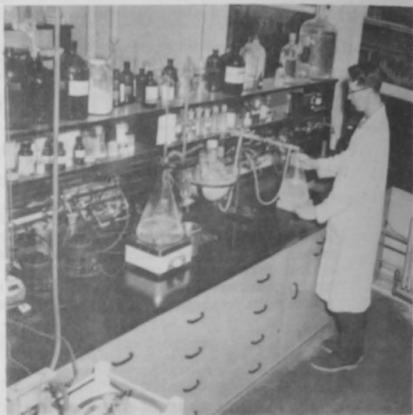
Fig. 2 - Simultaneous hydrolysis and steam distillation of sodium-reduction products of triglycerides, Seattle Technological Laboratory, Seattle, Wash.
