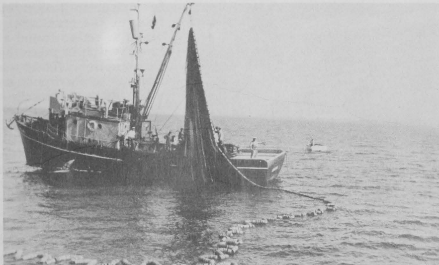
Fig. 6 - German-built steel-hull dragger converted for purse-seining in Turkish waters hauling in the purse seine.
