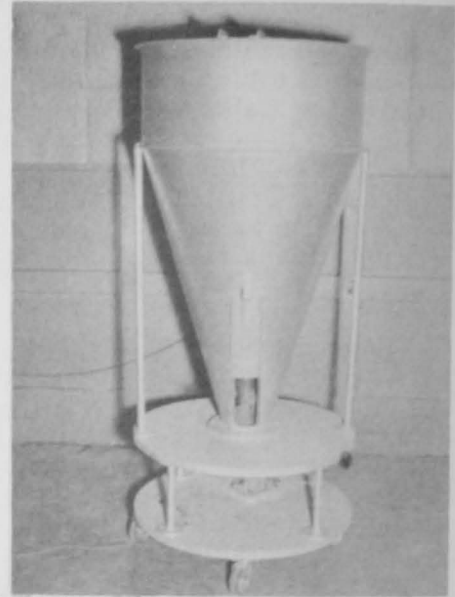
FIG. 1 - THE PORTABLE FISH-MEAL BLENDER, SHOWING THE SLIDE AT THE BASE FOR REMOVAL OF THE MEAL AFTER MIXING.
