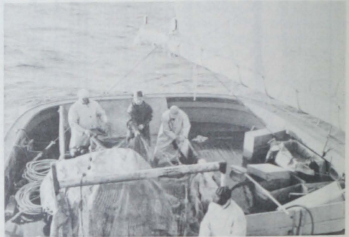
FIG. 4 - THE GILL NETS WERE PILED IN THE STERN BIN READY FOR SETTING AT THE NEXT STATION. THE SAIL WAS USED ONLY FOR STABILIZING EFFECT.
