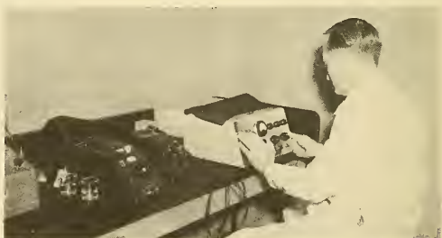
Fig. 1 - Measurement of color developed during browning reaction employing a differential type color instrument.
