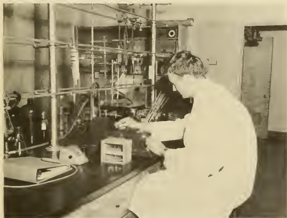
Fig. 1 - Colorimetric determination of tocopherol in king salmon oil.
