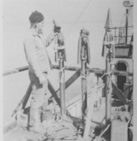
Fig. 15 - Engineer of the Dennis Gayle demonstrates how the bomb is screwed onto the harpoon. The harpoon in the center shows what is left after the bomb explodes in the whale.
