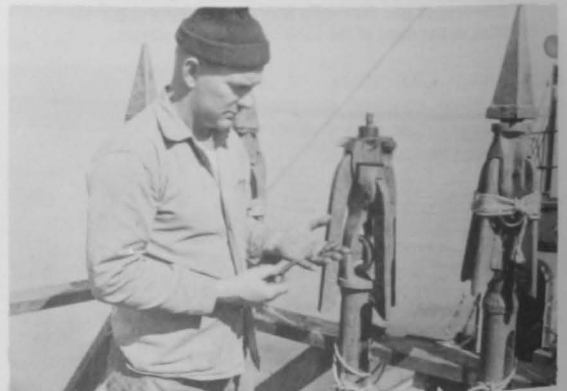
Fig. 17 - Parts of the fuse. The fuse has a plunger, which is the small part at the center of the engineer's hand. When the gun goes off, the jar knocks the plunger against a cap at the bottom of the cylinder (by the engineer's thumb of his right hand), which ignites the powder in the plunger and in the head of the fuse. This powder requires about 5 to 10 seconds to burn. It then ignites the powder in the bomb head, which explodes and kills the whale. Note the method of inserting the fuse on the harpoon in front of the engineer.
