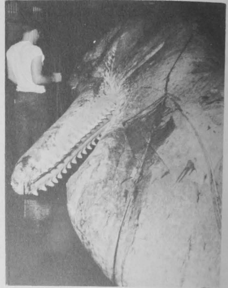
Fig. 23 - Cable-block. At the end of the cable in the worker's hand and hidden by the jaw of the whale is a block of wood. In removing a strip of the blubber, the worker chops a small hole in the end of the strip, which has been peeled from the whale for a short distance. The cable shown in the worker's hand is passed through this hole, and the block of wood at the end keeps the cable from going on through. The cable then is attached to a winch.
