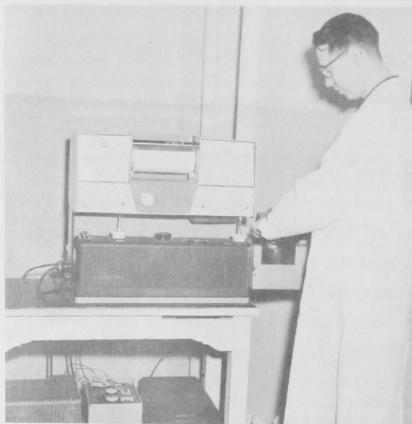
Fig. 1 - Ultraviolet absorption measurements being made on long-chain fatty alcohols used to prepare alkyl halides.
