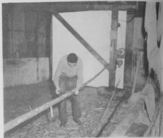
Fig. 8 - Preparing set-net stakes for stationary gill nets. These stakes must be peeled and sanded. Otherwise the nets will catch on the bark and tear in the swells. The stakes are about 35 feet long and are made from hemlock poles obtained at Sand Lake, which is 18 miles from Bay City. The building shown here is the end building on the right in fig. 6.
