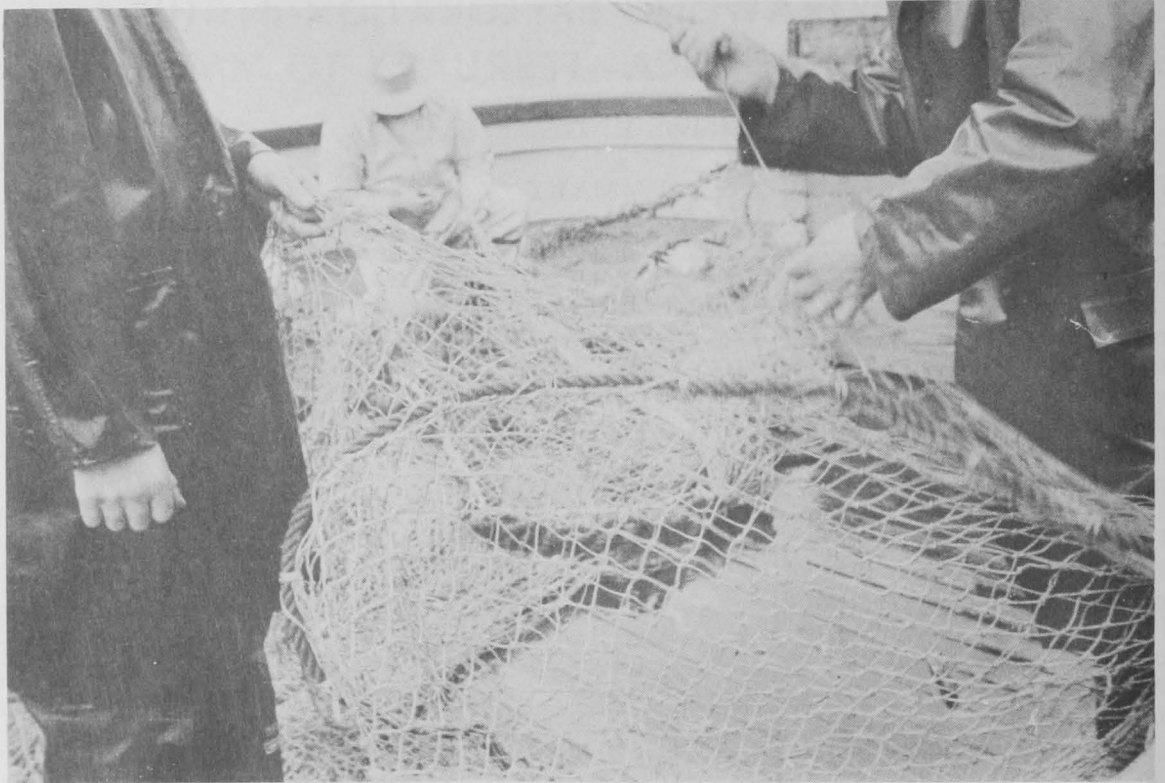
FIG. 2 - MENDING THE OTTER TRAWL ABOARD THE JOHN N. COBB WAS A FREQUENT CHORE, RESULTING FROM THE ROUGH BOTTOM IN MUCH OF THE STRAIT.
