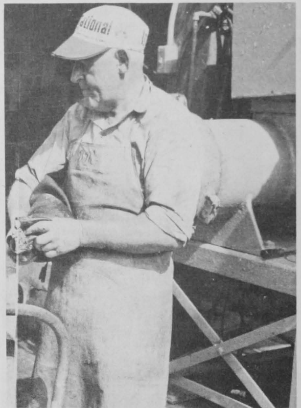
Fig. 11 - Extruder. After the anchovies pass through the hasher plate, they are extruded from this rubber inner tube. The purpose of the inner tube is to speed up the bag filling. As one bag is filled, the end of the tube is pinched and moved to the next bag in the line. When the bags on one side of the cart are filled, the cart is reversed, and the operation is continued without loss of motion.
