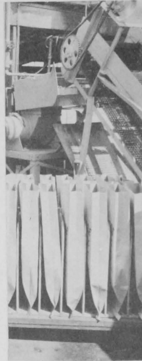
Fig. 10 - Multiwall paper bags and cart. The bags are 13x4x31 inches in size, and each one accommodates 50 pounds of groundfish. The inner wall of the bag is 60-pound, wet-wax, wet strength. The outer wall is 50-pound, natural kraft paper printed to indicate the type of fish, the size of grind, and the date the fish were placed in the freezer. The printed bag eliminates hand stenciling and thereby reduces labor costs. The carts hold 16 bags, totalling 800 pounds of ground fish when the bags are filled. Note that the bags are inserted into a partitioned plywood frame that prevents sagging of the bags and provides a uniform package. The frame is removable from the cart for cleaning purposes.
