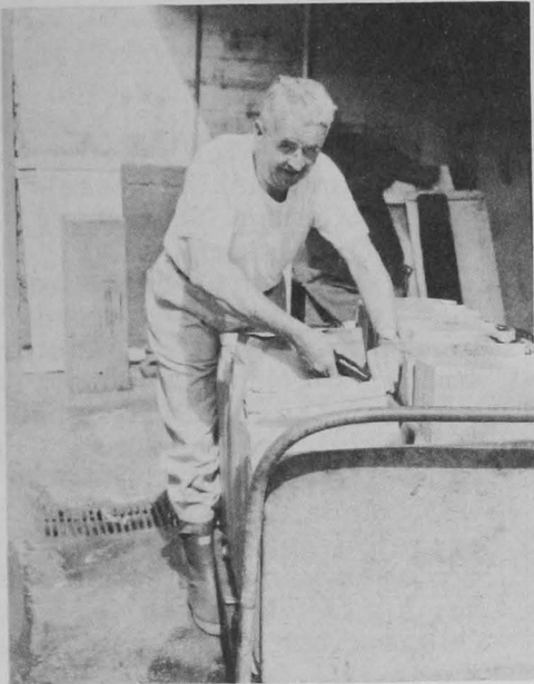
Fig. 12 - Closure of bags. The tops of the bags are folded double and are fastened with four staples across the top. As the bags on one side of the cart are filled, those on the other side are stapled.
