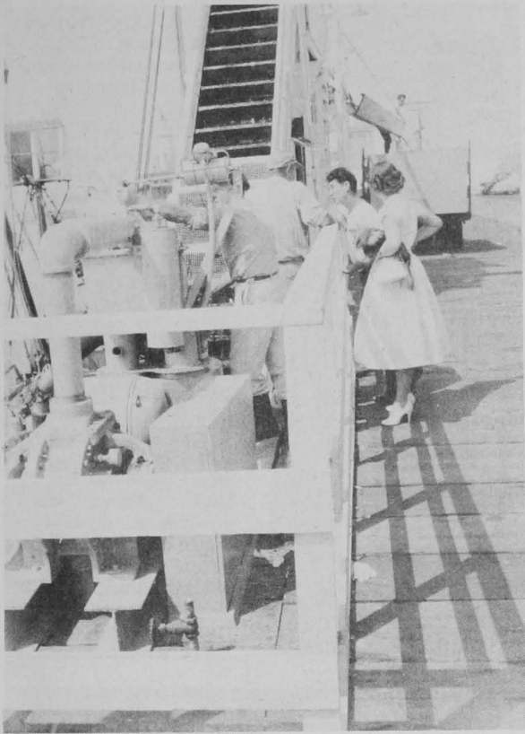
Fig. 3 - Pump and pump operator. This suction pump has an unloading capacity of 3,200 pounds of anchovies per minute. The pump is operated by a 40-horsepower 220-volt electric motor actuating a vacuum pump producing 25 inches of vacuum.
