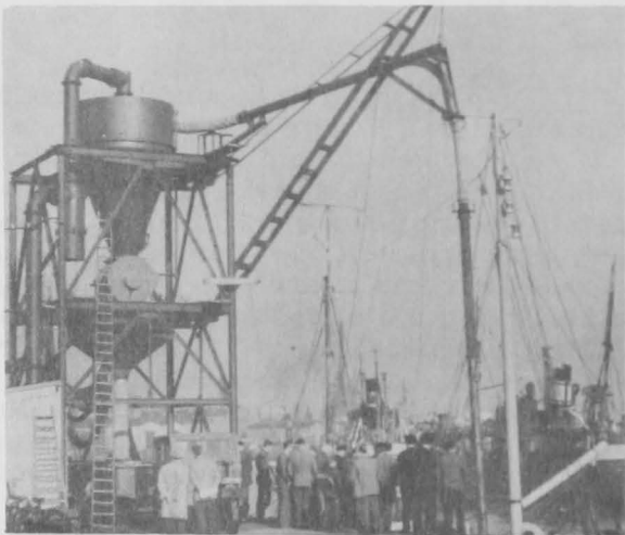
Fig. 2 - Shows pneumatic fish discharger set-up to unload fish directly from a vessel.
