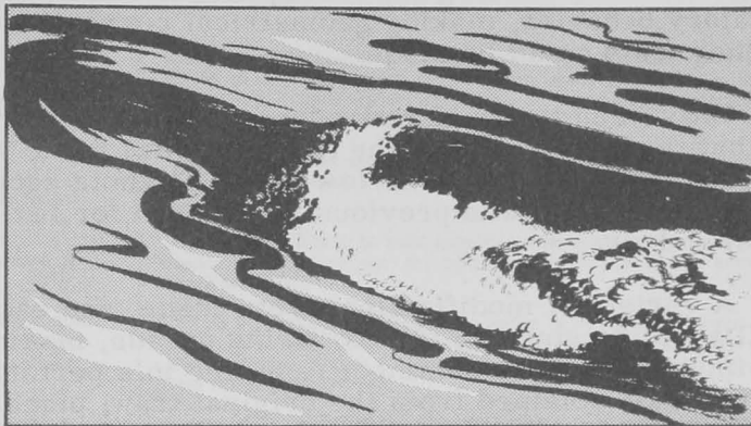
FIG. 3 - HYDRODYNAMIC TESTS OF ORIGINAL TRAWL PLANE FLOAT REVEALED THAT THE DRAG FACTOR WAS EXCESSIVE AND OVERCAME UPTHURST AT SPEEDS OF TOW ABOVE 3 KNOTS. SKETCH SHOWS VORTEX CREATED BY DRAG IN THE ORIGINAL MODEL OF THE WEIGHTED PLANE BEING TOWED IN A SWIMMING POOL.
